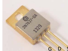
TO – 257 (Isolated Base-plate Hermetic Package)
