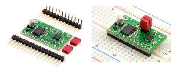
The qik ships with a 16×1 straight 0.100" male header strip, a 12×1 right angle 0.100" male header strip, and two red shorting blocks. This hardware offers several options when it comes to making connections to the qik.
