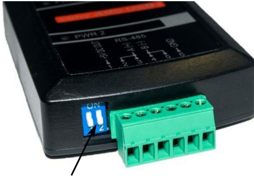
DIP-switch ON: RS485 termination connected
