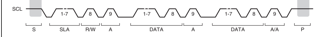
Figure 14.5 I 2 C Bus Timing
