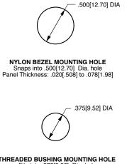
THREADED BUSHING MOUNTING HOLE Fits into .375[9.52] Dia. hole Bushing Length: .312[7.92]
