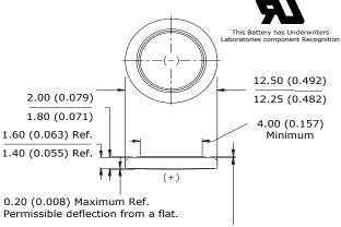
0.03 (0.001) Minimum Ref. (Applies to top edge of gasket or edge of crimp, whichever is higher.)
