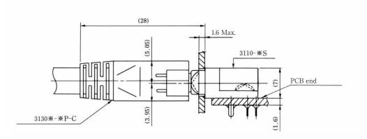
Note: Screw for Panel: M3×0.5 length 6mm.
