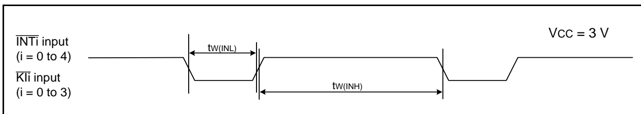
Figure 33.15 Input Timing Diagram for External Interrupt \overline{INTi} and Key Input Interrupt \overline{Kli} when V_{cc} = 3 V
