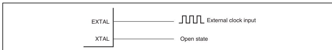
Figure 4.4 Example of External Clock Connection
