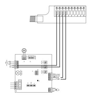
Fig. 2. Example of the connection of one channel of the Proxi Gate module to the gate controller (Beninca JM3 controller)
