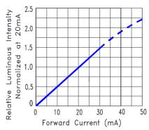
Fig.4 Relative Luminous Intensity vs. Forward Current
