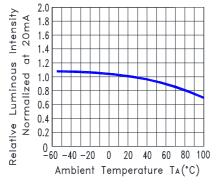
Fig.5 Relative Luminous Intensity vs. Ambient Temperature
