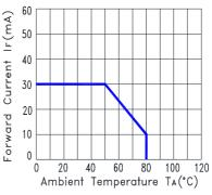
Fig.2 Forward Current Derating Curve
