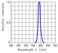
Fig.1 Relative Intensity VS. Wavelength
