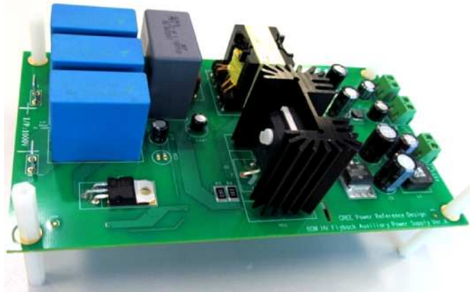
Figure 3: Photo of 60W auxiliary SMPS with 1700V SiC MOSFET
