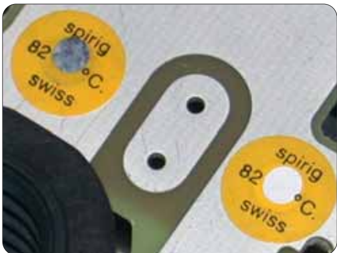
CelsiPoint® with one 82°C level. CP on left side exceeded and on right side never exposed to or above 82°C.
