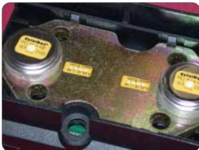
CelsiDot® 's with 93°C level and MICRO-CelsiStrip® s on an assembly before test.
