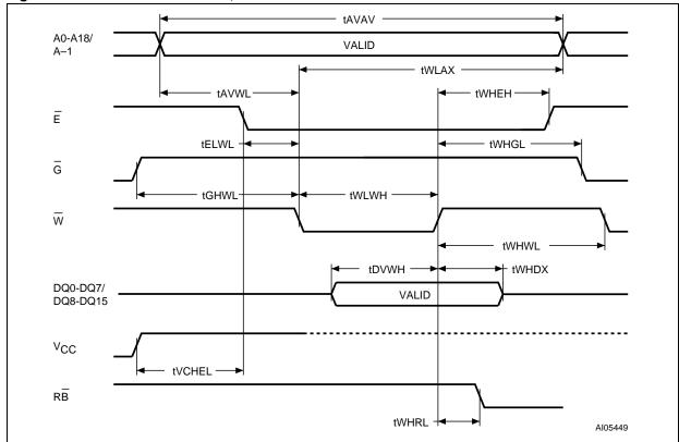
Figure 12. Write AC waveforms, write enable controlled
