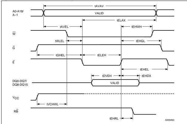
Figure 13. Write AC waveforms, chip enable controlled
