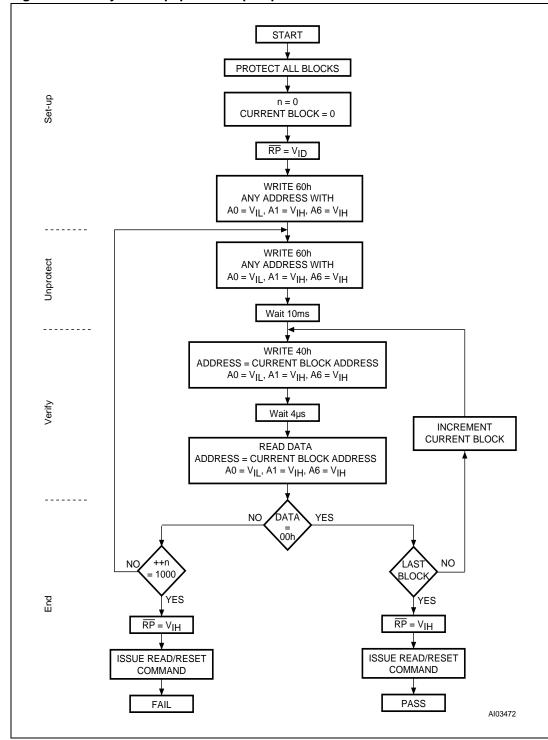
Figure 21. In-system equipment chip unprotect flowchart
