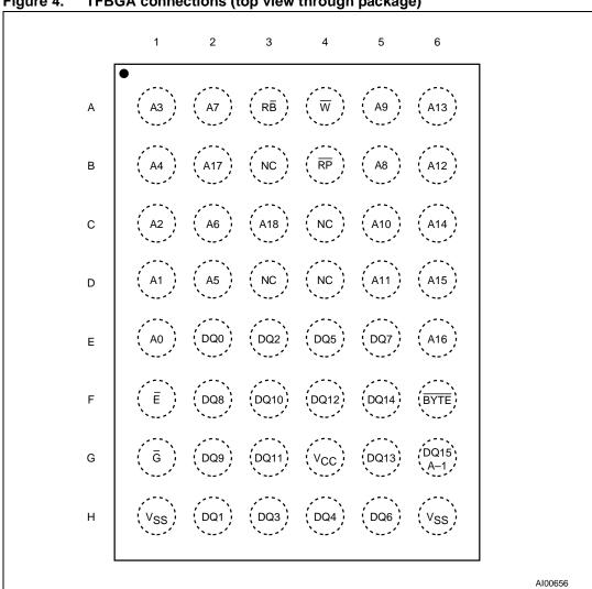
Figure 4. TFBGA connections (top view through package)
