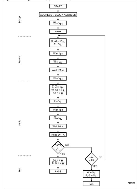
Figure 18. Programmer equipment block protect flowchart
