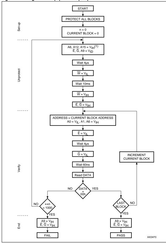
Figure 19. Programmer equipment chip unprotect flowchart
