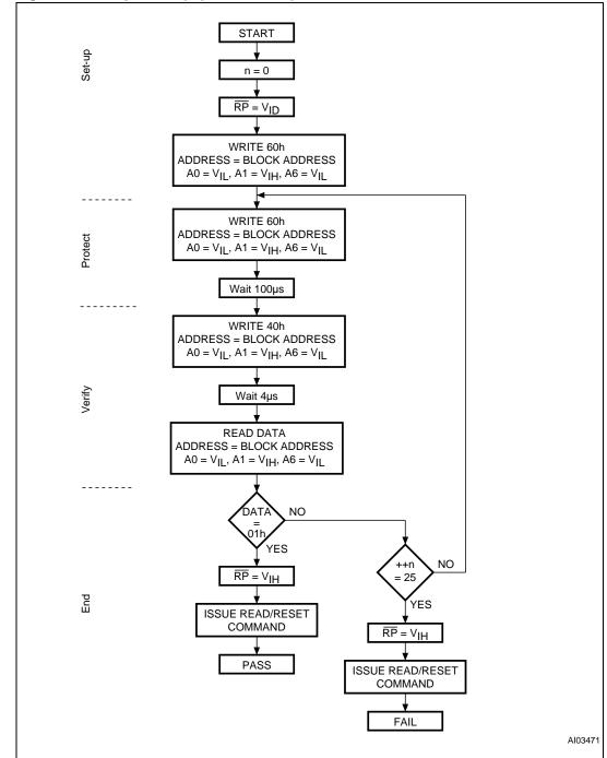
Figure 20. In-system equipment block protect flowchart
