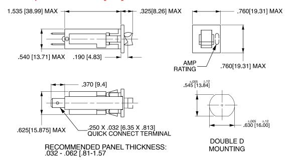
All dimensions are in inches [millimeters]. Tolerance  $\pm$ .005 [.127] unless otherwise specified. Breaker must hold 100% of rated current and must trip at 150% and above, within the time limits shown in curve. Trip times specified at 25° ambient with no preloading.
