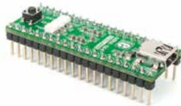
MIKROE-1368 MINI-M4 for Stellaris contains LX4F230H5QR (ARM ® Cortex ™ -M4)
