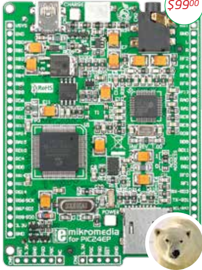
mikromedia for PIC24EP (features PIC24EP512GU810)
