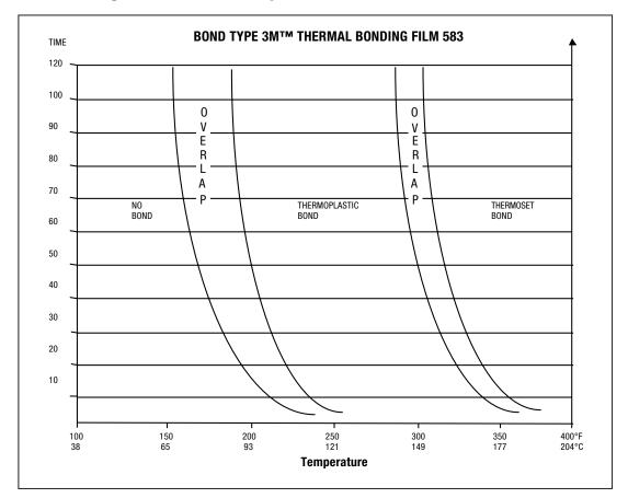
3M<sup>™</sup> Thermal Bonding Film 583 Bond Graphs
