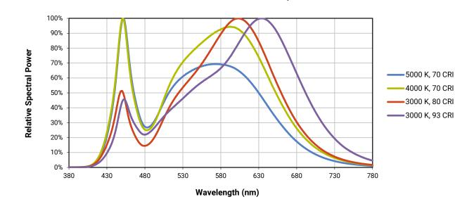
The following graph is the result of a series of pulsed measurements at 500 mA and  $T_{J}$  = 85 °C.
