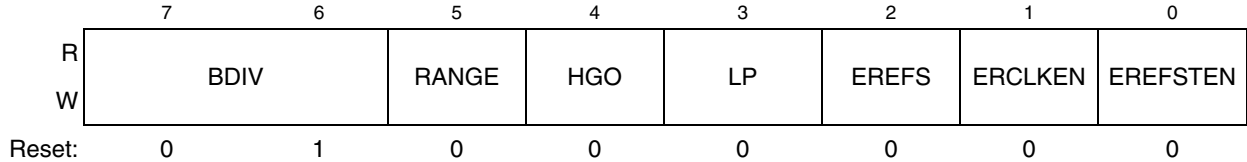
Figure 12-4. MCG Control Register 2 (MCGC2)
