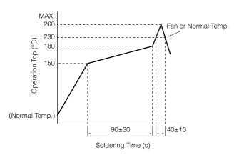
\*Reflow temperature may vary by location even in the same reflow condition. Please check the reflow temperature at terminals and at the top of a switch to make sure the both temperatures are withiin the specification. If even one of them is out of the specifications, please adjust.
