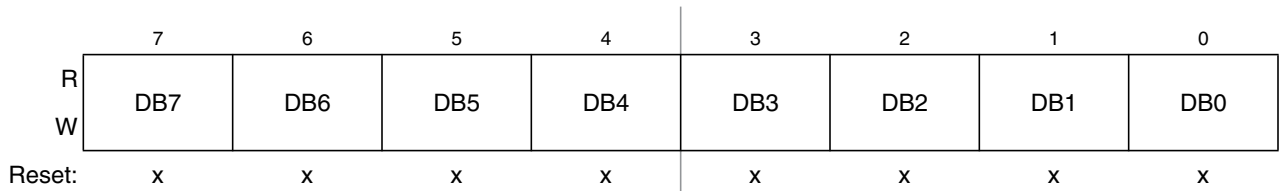
Figure 10-33. Data Segment Registers (DSR0–DSR7) — Extended Identifier Mapping
