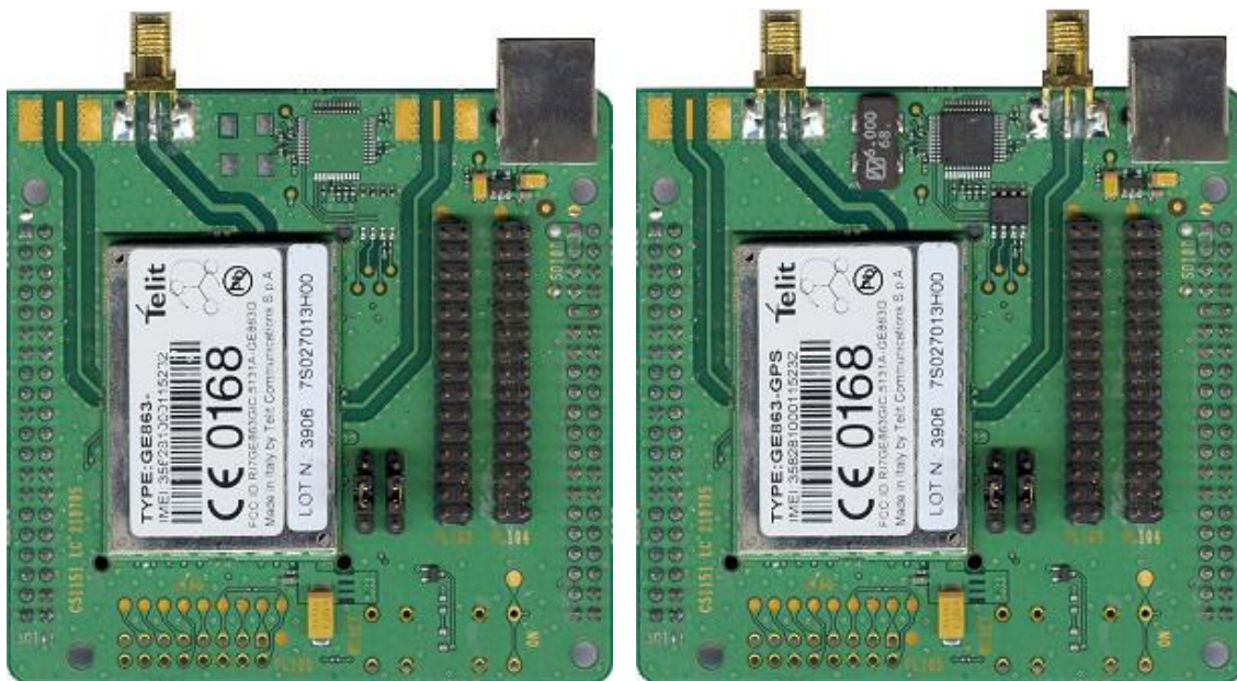
Figure 24. GE863 Interface Boards: GE863-QUAD or GE863-SIM (at left) and GE863-GPS (at right)
