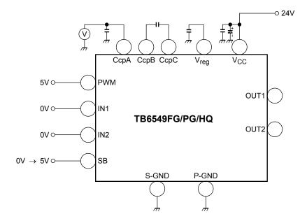
•  $tong: SB = 0 V \rightarrow 5 V$ . Measure the time taken to boost the CcpA voltage up to about 29 V (24 V + 5 V).
