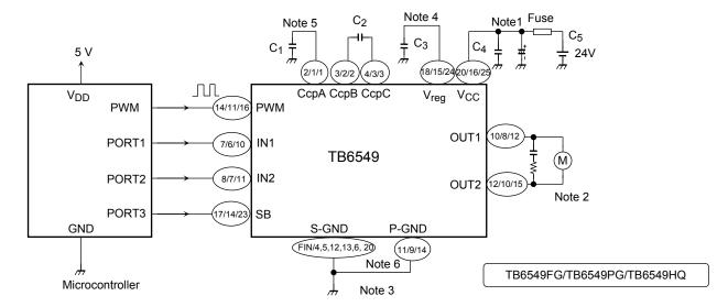
TB6549FG: Pins 1, 5, 6, 9, 13, 15, 16, and 19 are not connected. TB6549HQ: Pins 4, 6, 8, 9, 13, 17, 18, 20, 21, and 22 are not connected.
