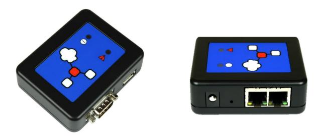
TCPConv adds a device, which is equipped with a USB- or RS232-interface into your local area network (LAN). A typical application is the extension of a network device (i.e. a network printer) by a local peripheral device. Simply insert TCPConv into the existing LAN connection of your device. In order to do so, TCPConv contains 2 LAN ports, which operate as a network switch.
