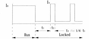
3rd wire signal Run : Square Wave Locked : VH or VL
