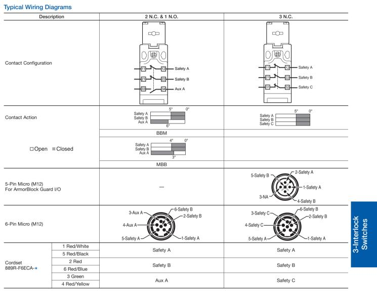
\* Replace symbol with 2 (2 m), 5 (5 m) or 10 (10 m) for standard cable lengths.
