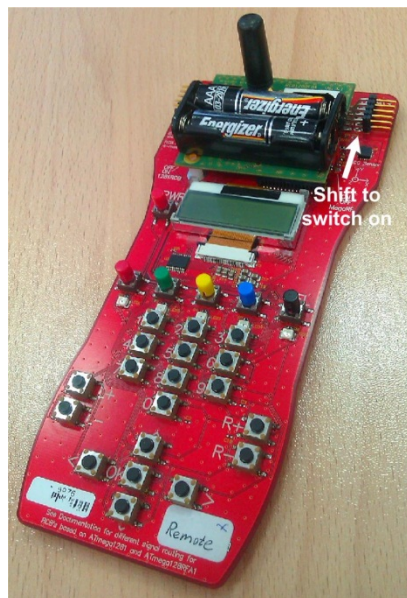
Figure 7-4. Assembled RCB Hosted on a Key Remote Control Board
