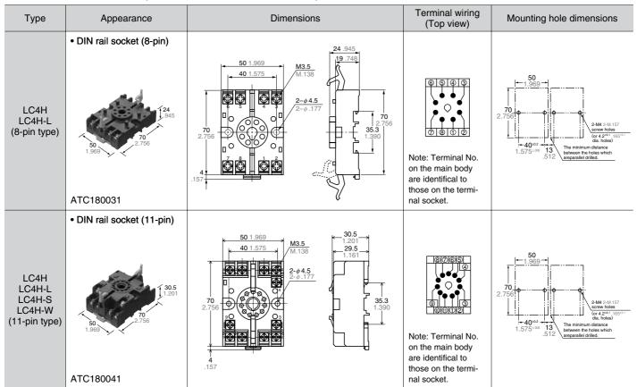
Note: The terminal numbers on the counter are identifical to those on the terminal socket.
