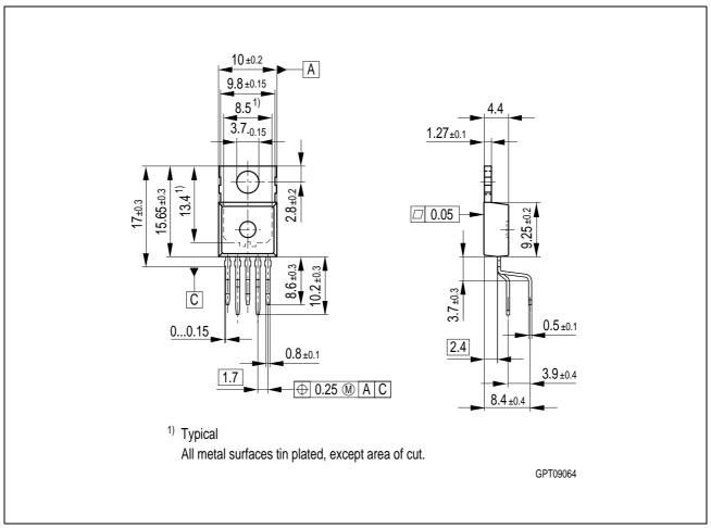
Figure 5 PG-TO220-5-11 (Plastic Transistor Single Outline)
