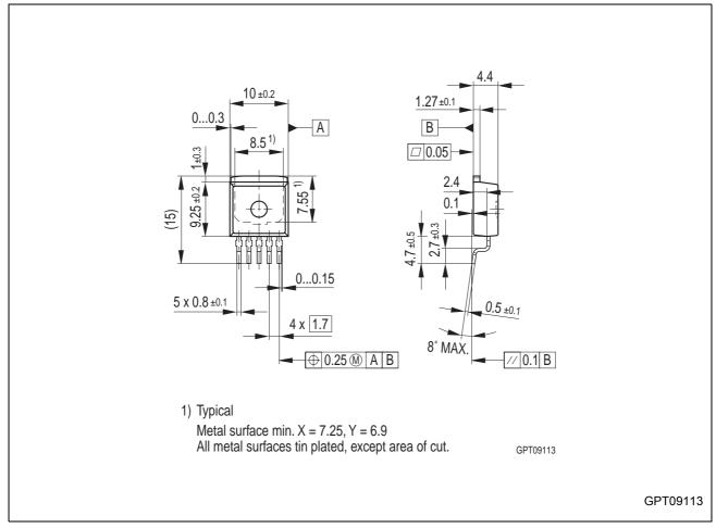
**Figure 7 PG-TO263-5-1** (Plastic Transistor Single Outline)
