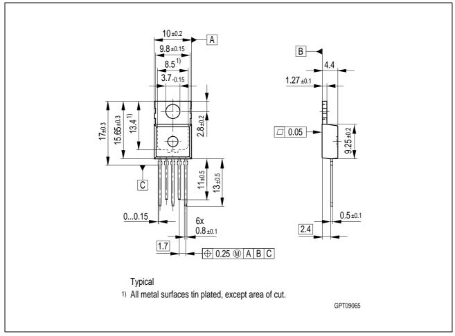
Figure 8 PG-TO220-5-12 (Plastic Transistor Single Outline)
