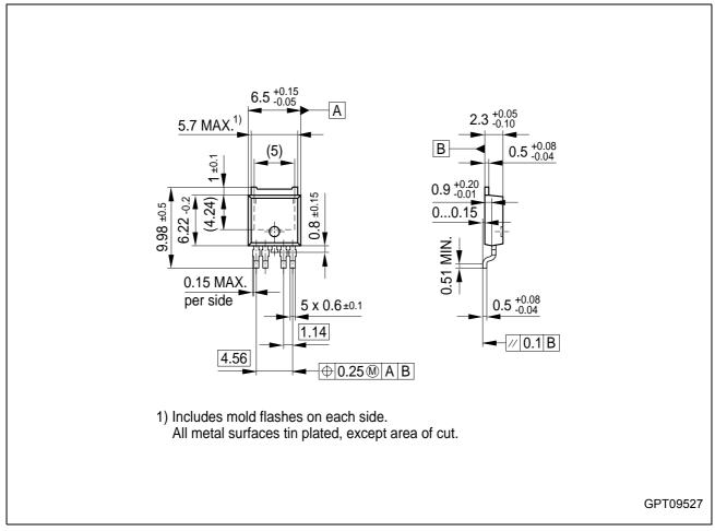
**Figure 6 PG-TO252-5-11** (Plastic Transistor Single Outline)
