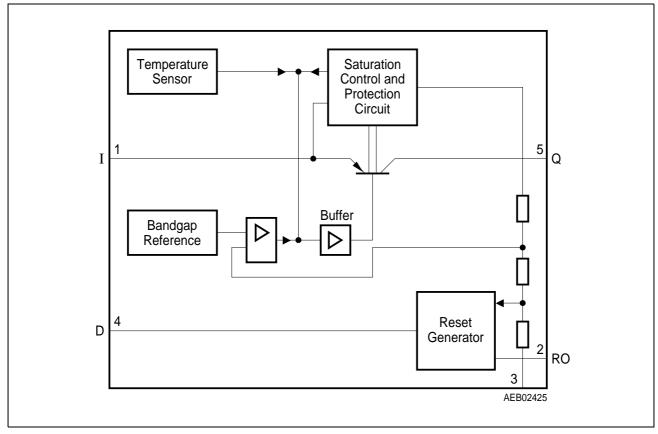
Figure 2 Block Diagram
