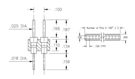
**Description:** Interconnect Header Solder Tail Pin Header .025" (0,64mm) Pin Head Double Row Through Hole Plating Code:
