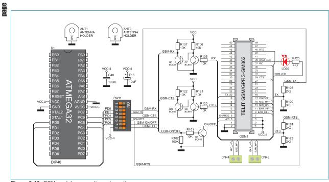
Figure 9-10: GSM module connection schematic
