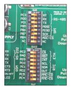
To connect a memory card to the microcontroller, it is necessary to set switches 4, 5 and 6 on the DIP switch SW9, as well as switches 7 and 8 on the DIP switch SW10 to the ON position.
