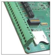
Figure 11-1: A/D inputs' connectors
