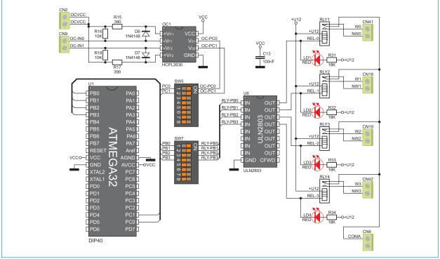
Figure 12-3: Relays and optocouplers and microcontroller connection schematic
