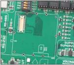
Figure 9-1: GSM connector
