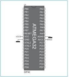
Figure 2-2: Microcontroller's pinout
