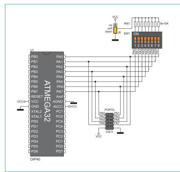
Figure 13-4: Port PORTA connection schematic
