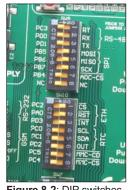
Figure 8-2: DIP switches SW9 and SW10
