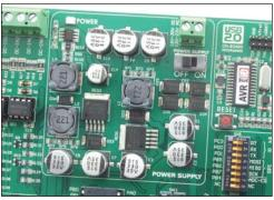
Figure 1-2: Power supply voltage regulator
