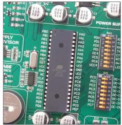
Figure 2-1: ATMEGA32 microcontroller
