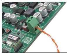
Figure 1-1: Providing power supply voltage
