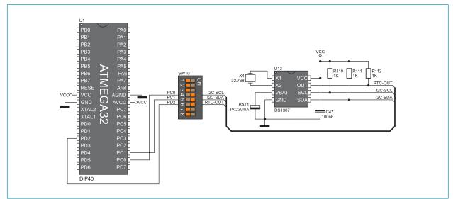
Figure 10-3: RTC module connection schematic
