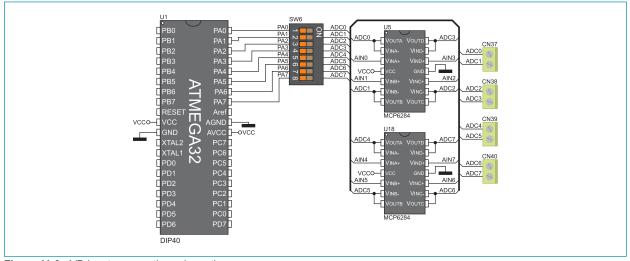
Figure 11-3: A/D inputs connection schematic
