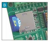
Figure 4-2: Inserting MMC/SD card
