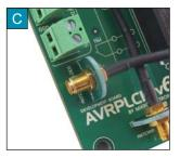
Figure 9-4: Screwing cable into antenna holder
