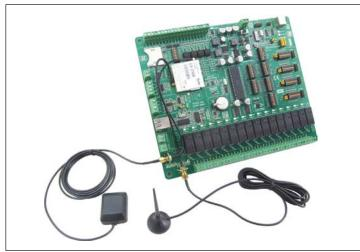
Figure 9-6: Telit's module with connected antennas
