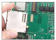
Figure 9-2: Connecting Telit's GM862 module
