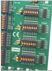
Figure 13-1: I/O ports
