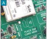
Figure 9-7: Inserting SIM card
