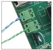
Figure 9-8: Connectors used to connect microphone and speaker
