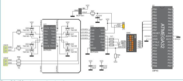
Figure 7-5: ADC module connection schematic
