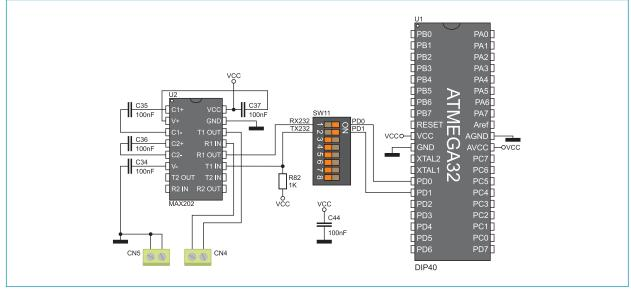
Figure 6-4: RS-232 module connection schematic
