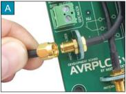
Figure 9-5: Connecting antenna
