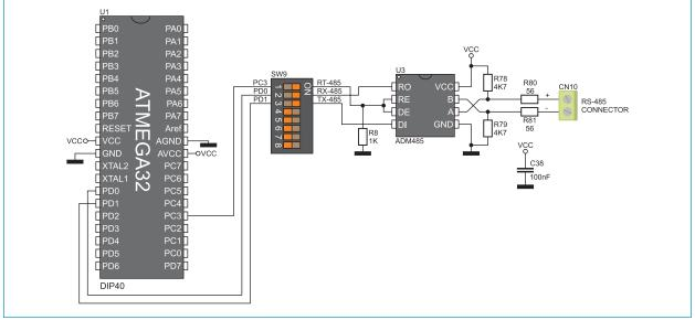
Figure 5-4: RS-485 module connection schematic
