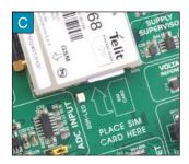
The GSM module gives a possibility of making phone calls. To enable this function, it is necessary to connect a speaker to a screw terminal CN43 as well as a microphone to a screw terminal CN44. For more information refer to the Telit's GM862 datasheet. Calling number and other parameters referring to the GSM module are defined in the program loaded into the microcontroller.
