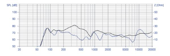
frequency response (1 W / 1 m) black = HDF board (690 x 660 x 4 mm) blue = MDF board (1200 x 800 x 19 mm)
