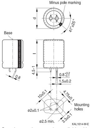
Snap-in capacitors are also available with 3 terminals (length (4.5-1) mm). PET insulation is marked with "PET" on the sleeve. Safety vent on the base.
