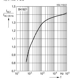
Frequency factor of permissible ripple current I<sub>AC</sub> versus frequency f  $V_R \ge 160 \text{ V DC}$
