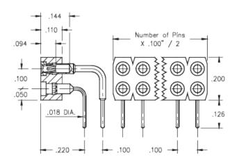
**Description:** Interconnect Socket Right Angle Socket Accepts .015" - .025" (0,38 - 0,635 mm) dia leads Double Row Through Hole
