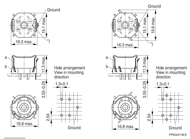
\*) This recess must be on the side of the grounding pin to ensure that the yoke locks in position.
