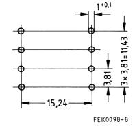
Hole arrangement View in mounting direction
