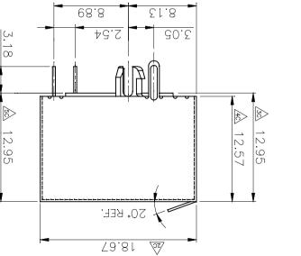
SHIELDED: BRASS WITH NICKEL PLATED. TIN PLATING OVER NICKEL IN SOLDER AREA. PLATING: GOLD PLATING OVER NICKEL IN CONTACT. CONTACTS: PHOSPHOR BRONZE. FLAMMABILITY RATING UL 94V-0.
