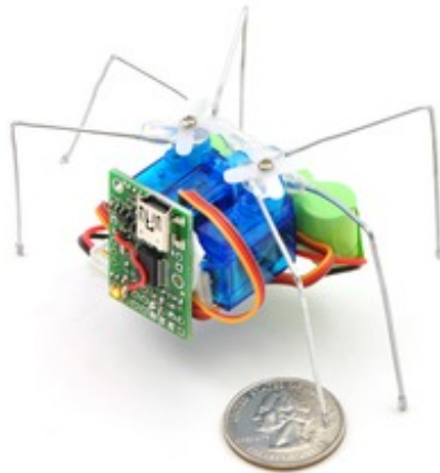
Micro Maestro as the brains of a tiny hexapod robot.
