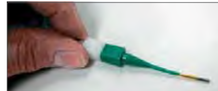
Plastic tool with contact in proper position.
