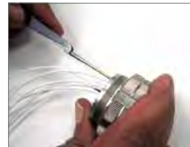
Removal of contacts with metal tool.
