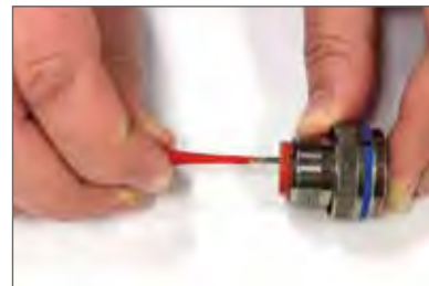
Plastic tool with contact in proper position.
