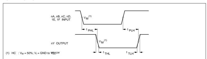
Fig.6 Waveforms showing the input (nA, nB, nC, nD, 1E, 1F) to output (nY) propagation delays and the output transition times.
