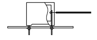
Temperature monitored inside the capacitor.
