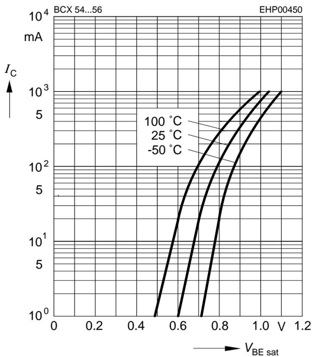
**Collector current  $I_C = f(V_{BE})$**
