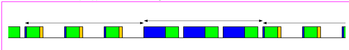
Figure 12: Extended PWM format with DUAL[5:1] = 01h (2 repetitions for each data)
