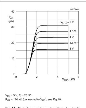
Fig.11 Gate 1 current as a function of gate 2 voltage; typical values.
