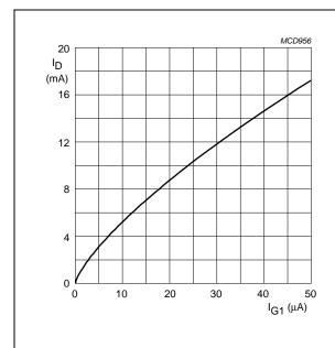
$V_{DS}$  = 5 V;  $V_{G2-S}$  = 4 V.  $T_j$  = 25 °C.
