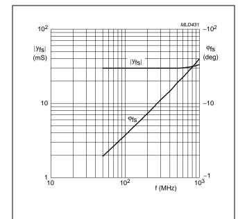
Fig 17 Forward transfer admittance
