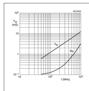
$V_{DS} = 5 \text{ V}; V_{G2} = 4 \text{ V}.$
