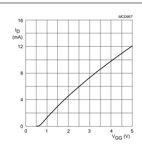
$V_{DS}=5~V;~V_{G2\text{-}S}=4~V;~T_j=25~^{\circ}C.$   $R_{G1}=120~k\Omega$  (connected to  $V_{GG});~see~Fig.19.$
