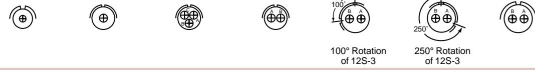
Front Face of Pin Insert or Rear Face of Socket Insert Illustrated
