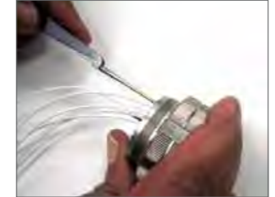
Removal of contacts with metal tool.
