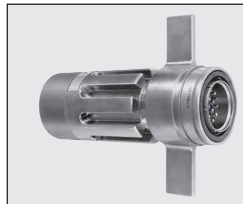
Special configuration Fail Safe used on space telescope application. Lanyard is replaced by a swivel ring for remote disconnect and "wing arms" have been added for manual actuation accessibility by gloved astronauts.
