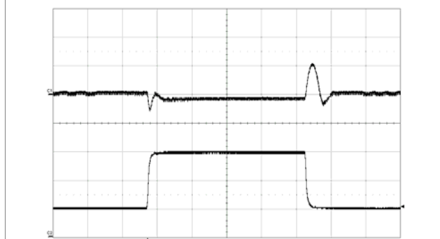
Output Load Transient Response, Default PID/NLR
