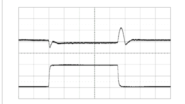
Output Load Transient Response, Default PID/NLR
