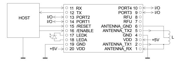
Connection diagram with external elements
