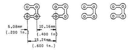
FIGURE 4 – PRINTED WIRING BOARD (TEST)
